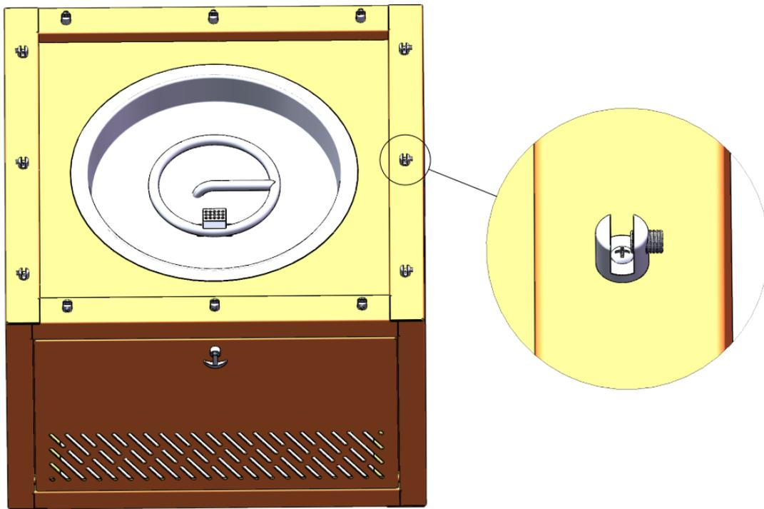
2. Insert glass to U shape hardware and screw horizontally to lock glass in place.
