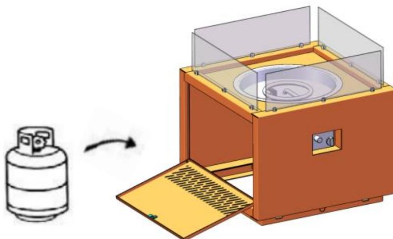
3. Turn the Cylinder Valve on the tank in a clockwise direction to TURN OFF SUPPLY of the LP Gas supply . Attach the preassembled Regulator from the Fire Table / Column to the Cylinder Valve by turning the Black Regulator Coupling Nut clockwise. Make sure it is fastened securely and tighten connections - by HAND only.
