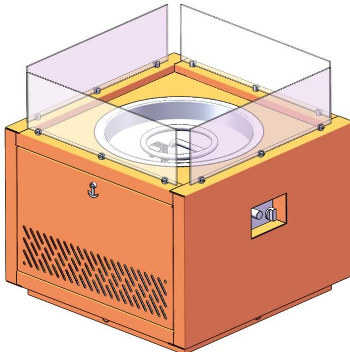
5. Remove the electronic igitor cap on operation tablet by unscrewing and slide AAA battery (not provided) into battery slot. Make sure the positive side of battery faces outwards. Screw the electronic igitor cap over battery tightly.
